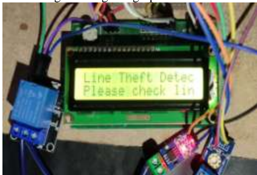
Step 4: Display to show Power theft detection at lineman side
