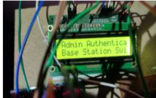
Step 5: Display to show admin authentication base station switching that is after entering the 4 digits password in keypad
